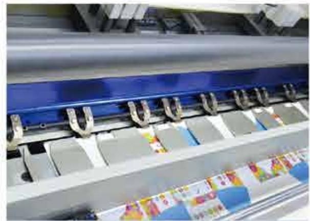
Double cam gripper bar system, offecct by KOMORI.
